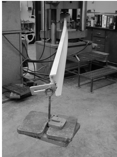
Figure 3 Experimental testing for lateral buckling of FRP channel shapes
