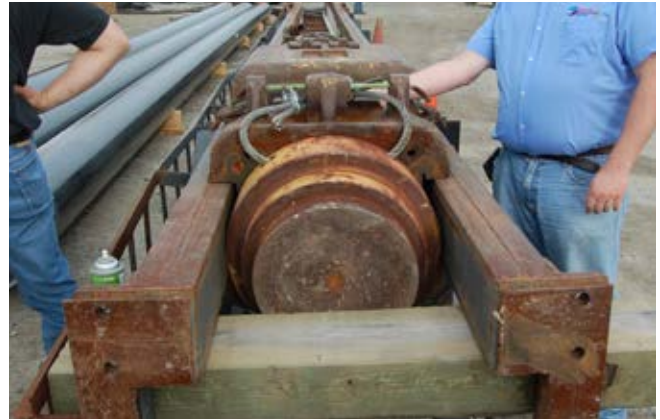
Pipe Insert Driving Head for Driving Hollow Piles
