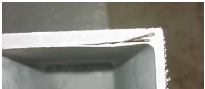
Example of Delamination in a FRP Square Tube
