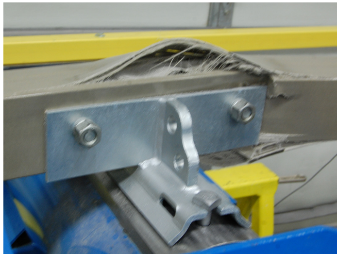
Figure 8: Minor-axis Bending Failure Mode
