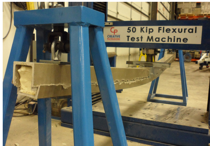
Figure 4: Typical In-plane Shear Failure at the Neutral Axis
