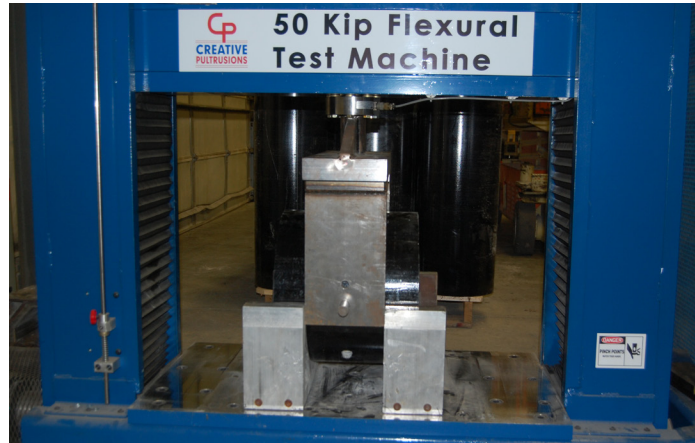
Transverse Pin Bearing Strength
