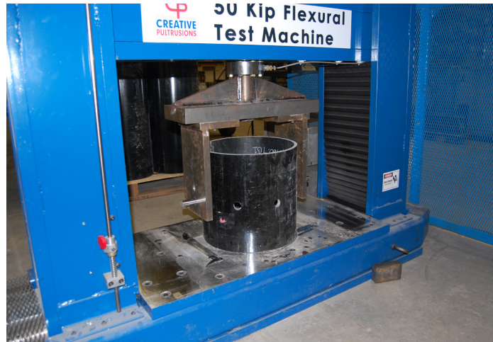
Lengthwise Pin Bearing Strength
