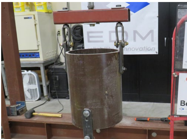
Bolt Bearing Testing at EDM International
