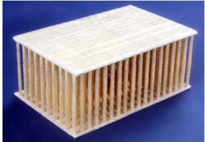
Close Up of the Fiber Insertions with the Core Foam Removed
