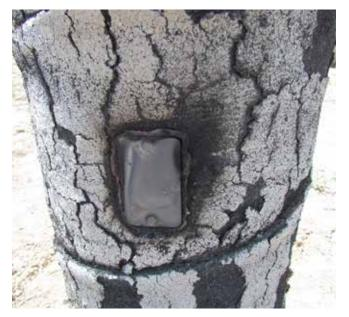
Post Fire Inspection Irreversible Temperature Measuring Device Access Cover Plate.
