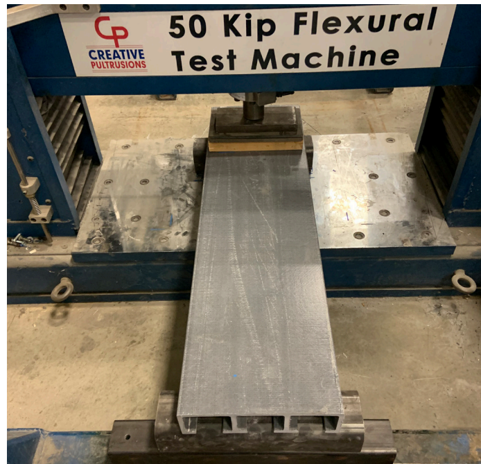
Figure 4: Schematic of GR120 H-5 deck shear load testing
