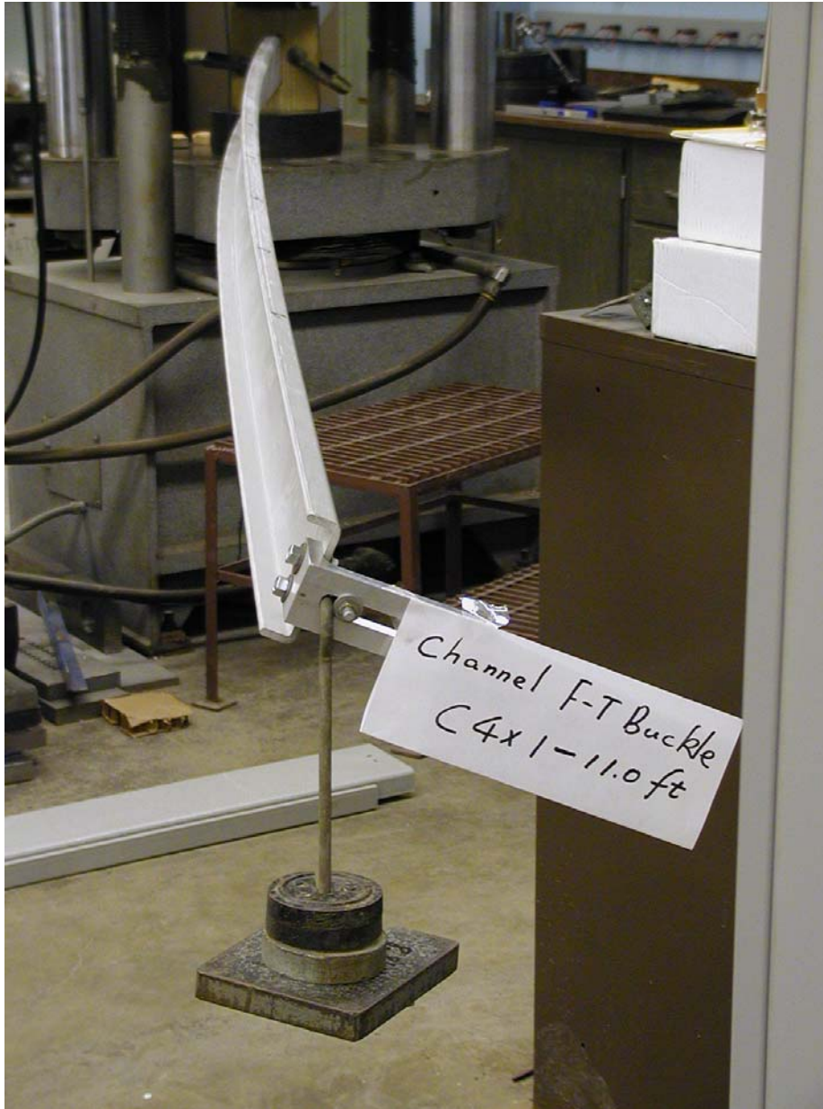
Figure 6 Buckled channel C4x1 beam ( L = 11.0 ft.)
