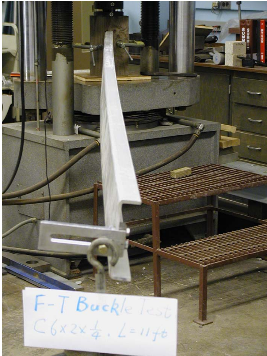
Figure 7 Buckled channel C6x2-A beam ( L = 11.0 ft.)
