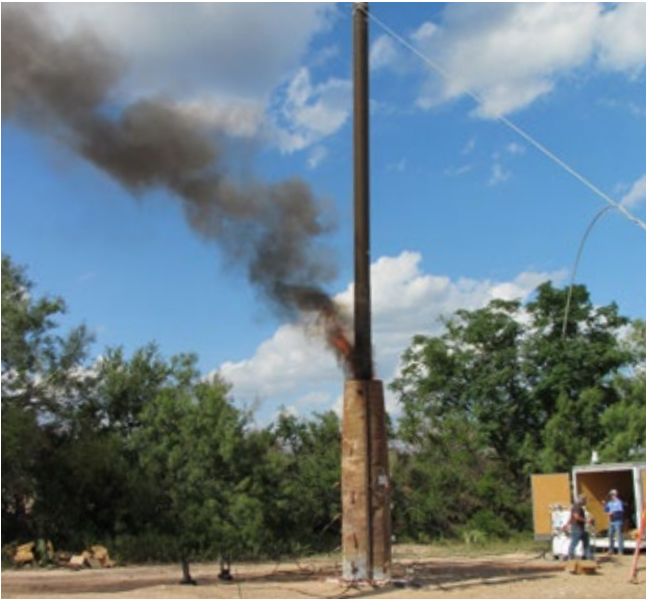
Fire Resistant Pole System being tested.
