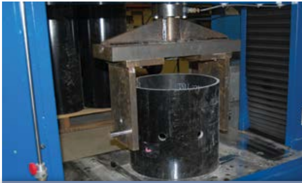
Bolted Connection Test - Parallel
