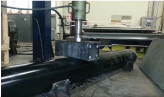
Crush Test on Concrete Filled Pile
