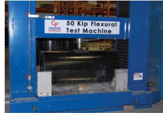
Pipe Pile Washer Push Pull Through Test Set Up
