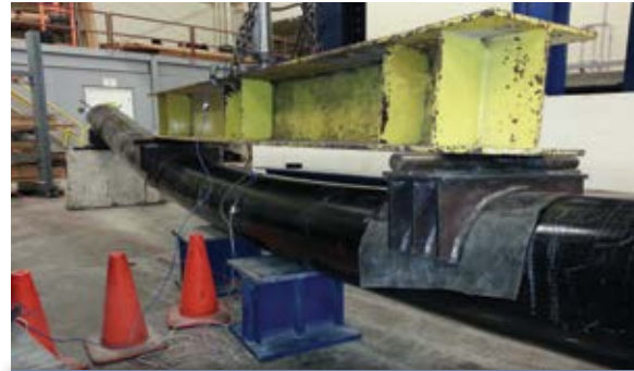
Full Section Testing of Concrete Filled Pile
