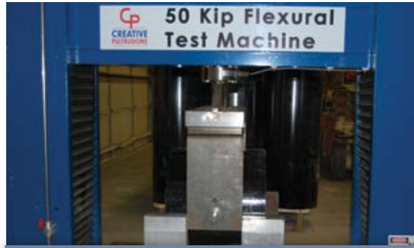
Bolted Connection Test - Perpendicular
